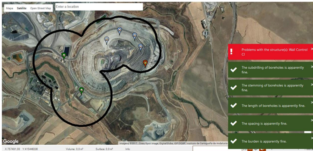
Fig. 303 – Detection of problems with the structures.
