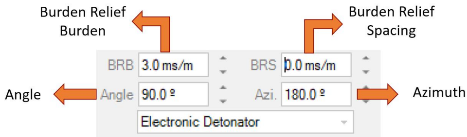
Fig. 226 – Parameters that change the direction vector
